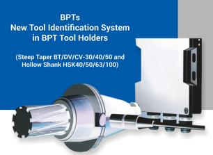
Data exchange between the data carrier and read/write head is non contact and therefore wear-free. The data and necessary power for the data carrier are inductively coupled by the read/write head. This means the data carrier requires no battery for power. The reliability of the data transmission is quaranteed by special checking software.
